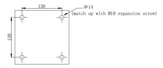
② Drill the Screw holes and twist the expansion bolts
